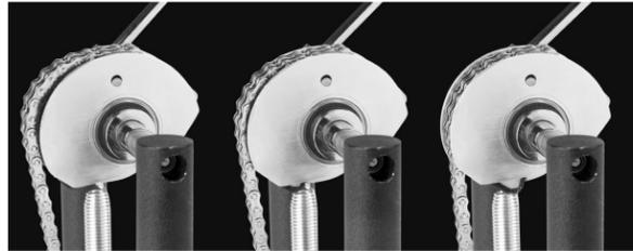
Torque position adjustments from eccentric (far left) to concentric (far right).
